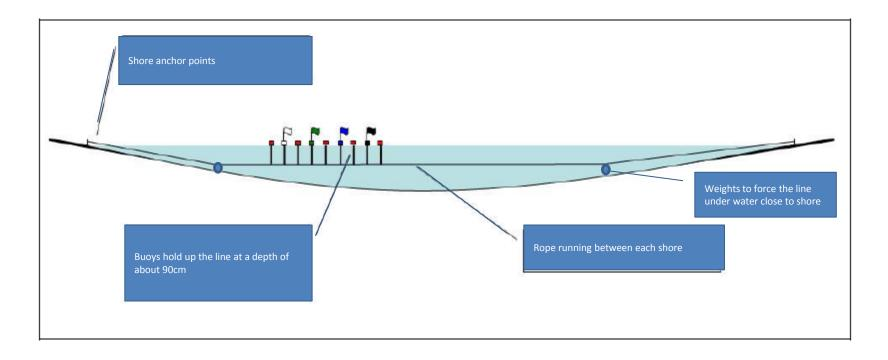
The set-up of the course is similar to setting up lanes in a swimming pool, albeit with the lines (rope or steel cable) running underwater, and only the buoys visible at the surface.
